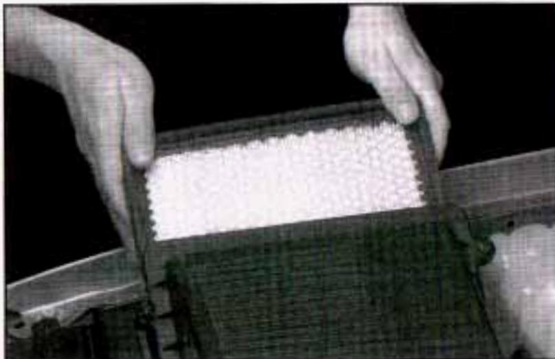
1. To remove the engine air cleaner/filter, loosen the screws on the cover.
