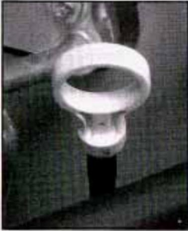
The engine oil dipstick has a yellow loop handle and is located in the engine compartment on the passenger's side of the vehicle. See *Engine Compartment Overview* on page 5-12 for more information on location.
