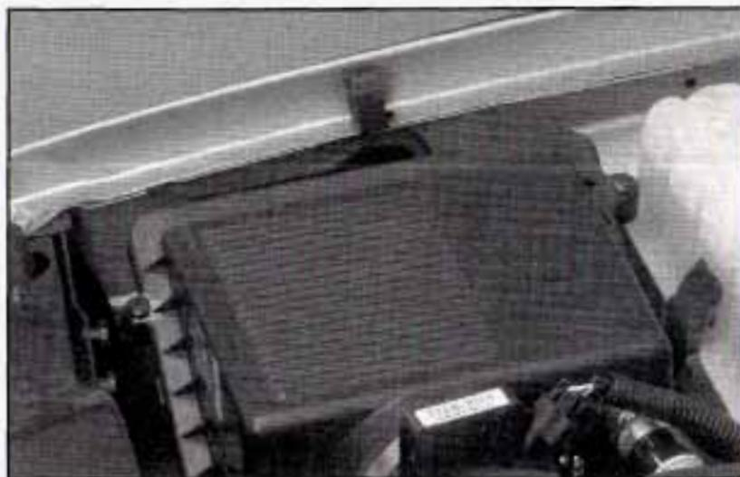
Your engine air cleaner/filter is located in the air filter housing near the front corner of the engine compartment on the passenger's side of the vehicle. See *Engine Compartment Overview* on page 5-12 for more information on location.
