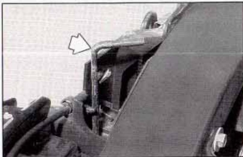
6. Remove the vertical pin from the headlamp assembly by turning the end of the pin away from you until it unsnaps and then pulling it upward.
