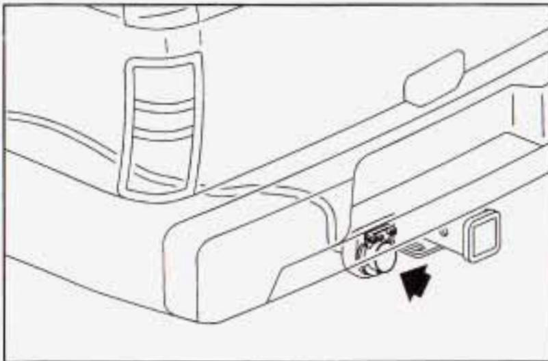
Your vehicle is equipped with the seven-wire trailer towing harness. This harness with a seven-pin universal heavy-duty trailer connector is attached to a bracket on the hitch platform.
