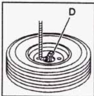
13. Tilt the retainer at the end of the cable and pull it through the wheel opening. Pull the tire out from under the vehicle.
