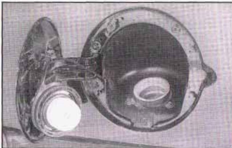
While refueling, hang the fuel cap by the tether using the hook located on the inside of the filler door. To remove the fuel cap, turn it slowly to the left (counterclockwise).
