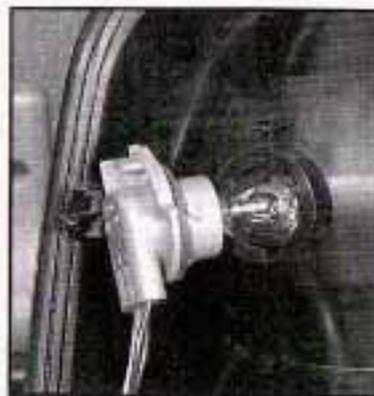
4. Pull the bulb straight out from the socket.
