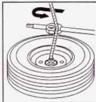
The wheel wrench has a hook that allows you to pull the hoist cable towards you to assist in reaching the spare tire.
