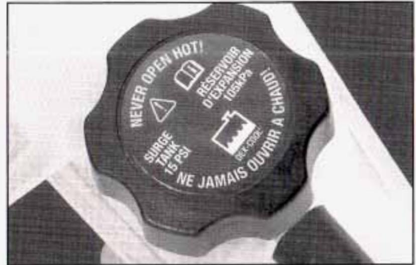
The coolant surge tank pressure cap must be fully installed on the coolant surge tank.
