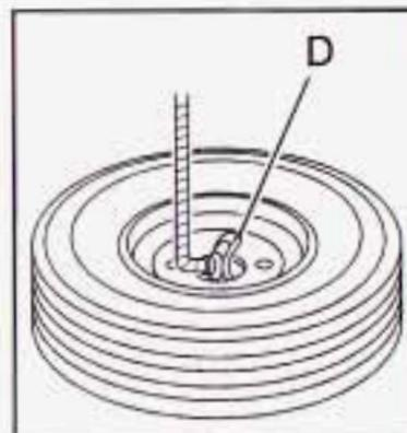
5. When the tire has been lowered, tilt the retainer (D) at the end of the cable so it can be pulled up through the wheel opening.
