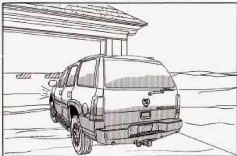
5. Turn the vertical aiming screw (V) until the headlamp beam is aimed to the horizontal tape line. The top edge of the cut-off should be positioned at the bottom edge of the horizontal tape line.
