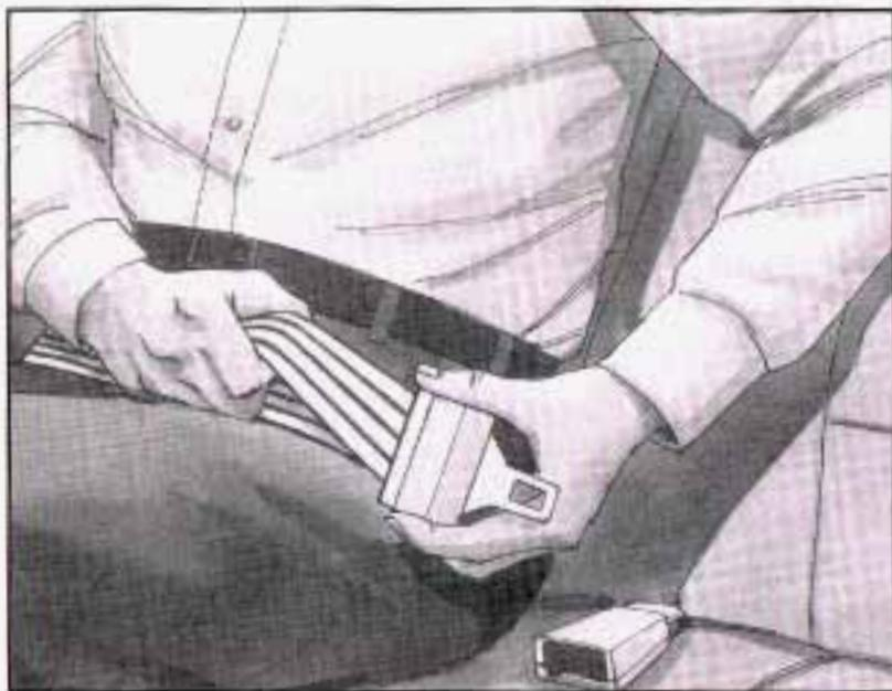
When you sit in the center seating position in the third row, you have a lap safety belt, which has no retractor. To make the belt longer, tilt the latch plate and pull it along the belt.
