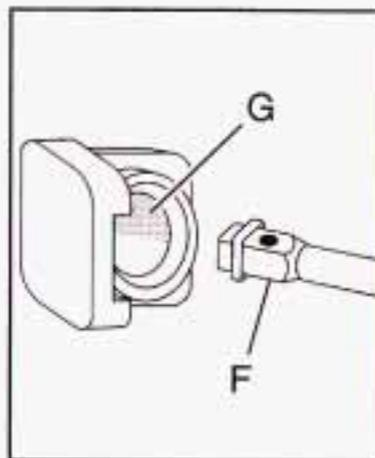
4. Insert the hoist end (F) through the hole (G) in the rear bumper and into the hoist shaft.
