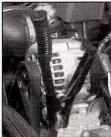
9. Connect the other end of the negative (-) cable at least 18 inches (45 cm) away from the dead battery, but not near engine parts that move.
