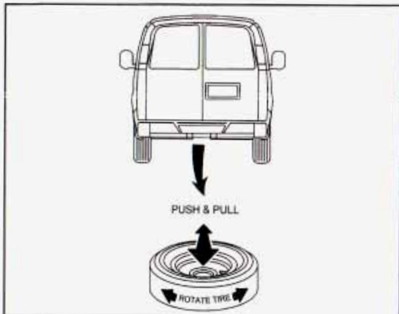
7. Make sure the tire is stored securely. Push, pull, and then try to rotate or turn the tire. If the tire moves, use the wheel wrench to tighten the cable. Reinstall the spare tire lock (if equipped).
