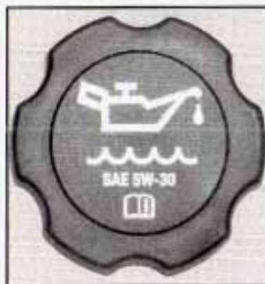
The engine oil fill cap is located on the valve cover on the passenger's side of the vehicle. See *Engine Compartment Overview on page 5-12* for further location information.
