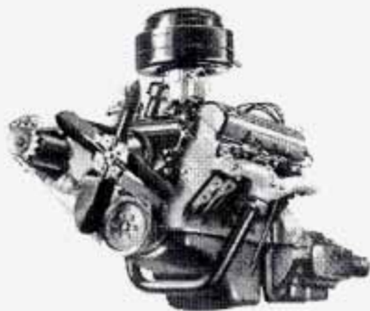
1949 Overhead Valve High Compression V8 Engine
