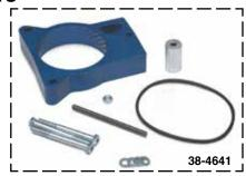
Powr-Flo Throttle Body Spacers are CNC-machined from billet aluminum and feature a bore engineered to increase velocity of airflow into intake manifold. This allows more air to reach combustion chamber for denser air charge and increase in fuel efficiency. The result is improved throttle response and power gains in mid-range and upper rpm operating ranges. Includes gaskets, hardware and instructions for a simple, bolt-on installation with no other vehicle modifications required.
