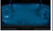
LED Cargo Lights provide great lighting and visibility with 8 LED modules (two 69" sets of four evenly spaced pre-wired LED modules). Each module has 6 super bright cool white LEDs and mounts easily below bed rail with pre-applied 3M™ tape and included wiring clips. Install with the included optional switch or wire into existing cargo light.
