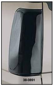
Tail Light Cover Set will dramatically enhance the look of your truck. Mounts easily using 3M™ Automotive Dual Lock, included. Brake lights show through when on, but disappear when off. Available in smoke only.
