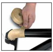
Increase performance by keeping hot exhaust gasses inside the headers for maximum velocity, improved exhaust scavenging and protecting sensitive engine components from high temperatures.
