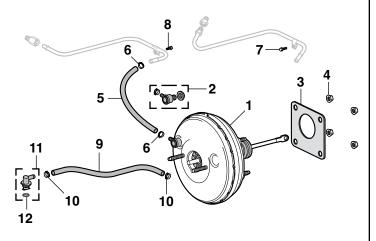
Core Refund Information - Brake Booster: A rebuildable core will have no excessive wear. No broken, cracked or dented housings. No worn or stripped threads. If it does not meet the above standards, it is not rebuildable and will not be refunded. DO NOT send a non-rebuildable core.
