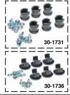
NotcHead Line Clamps organize both hard and soft lines and clamp them in place to keep from being chafed on sharp edges or crushed under moving components. Easily secure lines without marring paint. Can also be used as separators for running hoses in parallel by bolting two line clamps together. Flexible lines easily snap in for quick installation and mock-ups. Mounting hardware included in each kit.
