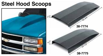
These 2" and 4" Universal Fit Hood Scoops are stamped from 18-gauge steel and coated with an Electro Deposit Primer (EDP) for a smooth surface. Installation will require cutting and forming the scoop to match the length and curvature of your truck's hood. Welding and body work will be required prior to painting.
