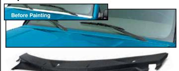
Replace that factory black grate between the hood and windshield with this simple urethane wiper cowl, making the hood flow all the way to the windshield. Comes complete with wiper and washer relief holes.
