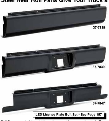
Roll Pans can eliminate stock rear bumpers for a smoother look. Easy installation. Finished with Black Electro Deposit Primer ready for painting. Check local bumper laws before ordering.
