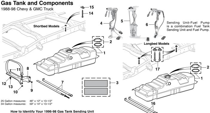
1996-98 models have a label attached to the wiring harness on the sending unit. The label has three letters printed on it that are referred to as the ID Code. Please order by matching the letters on your gas tank sending unit with the correct part number.
