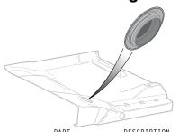
These flush mount Sheet Metal Plugs close unused holes in firewalls, floor pans and doors. Plugs are made of plastic and easily snap into 14 to 26 gauge sheet metal. Available in multiple sizes to fit 3/8" to 1" diameter holes.
