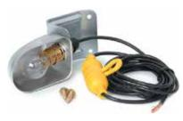
Underhood Lamp Kit adapts to any 12 volt truck and helps illuminate the engine bay. Necessary installation hardware is included. No need for wiring to a switch, bulb socket base is gravity activated; lamp comes on when hood is raised and goes out when lowered. Mount underneath hood and
