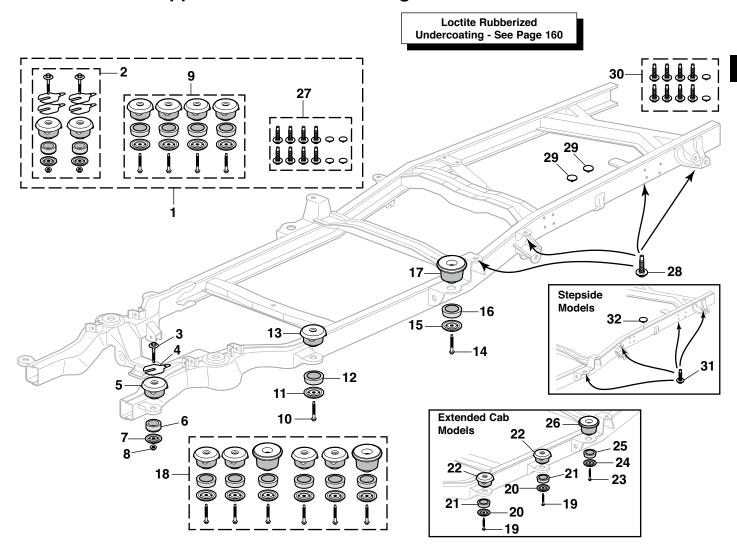
The Complete Mounting Kit includes the Radiator Core Support Mounting Kit, Front and Rear Cab to Frame Mounting Kit and the Bed to Frame Mounting Kit. These rubber cushions are made like original and provide a smooth ride while maintaining proper cab-to-bed alignment.
