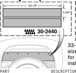
Body Gap Filler Set covers the gap between the frame and the bed of the truck. Body Gap Filler Set creates a clean backdrop for your wheels and is also used to cover the opening created by a body lift kit. Made from 3/16" thick industrial rubber, each piece measures 33-1/2" long by 4-3/4" wide and must be sized and cut to fit. Drilling is required for installation. Mounting hardware and
