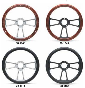
These 14" diameter, 3 spoke steering wheels have a half-wrap design featuring a billet back with a wood or leather grained vinyl front. Facing ring is available in hand-rubbed wood or black leather grained vinyl.
